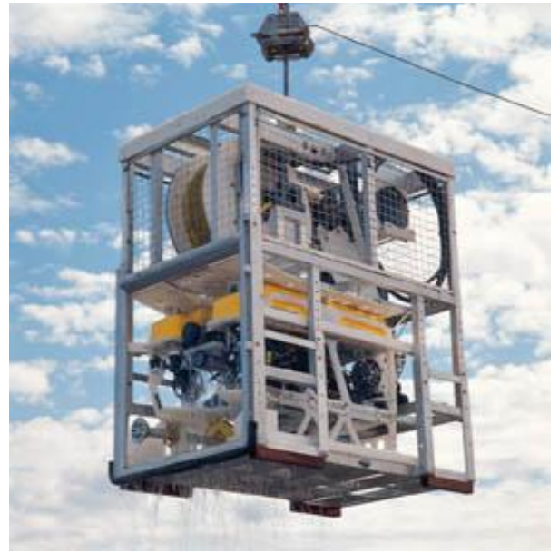
SeaEye Lynx with FMD orientation skid in a Seaye Winch and slip ring TMS
