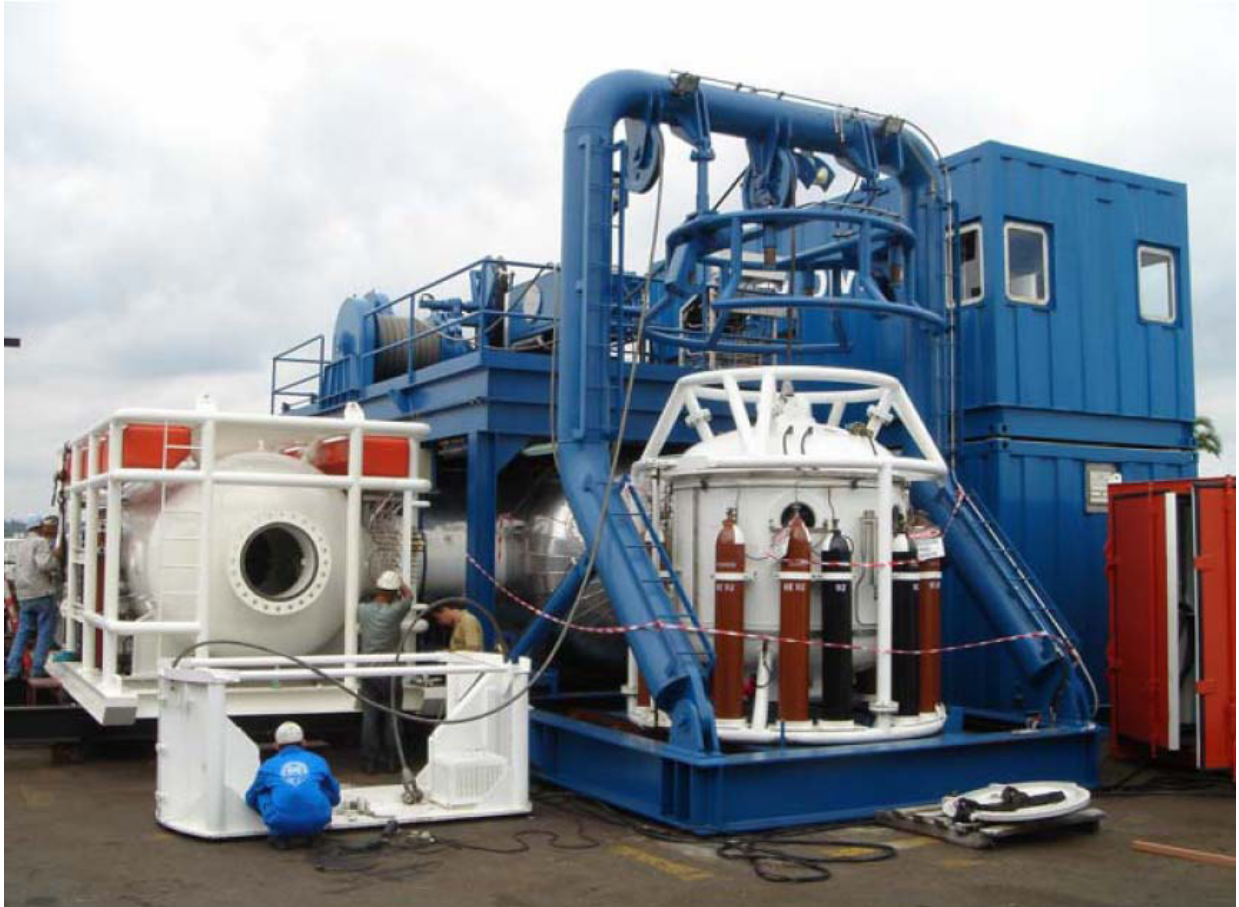
12- Man Saturation Diving System
